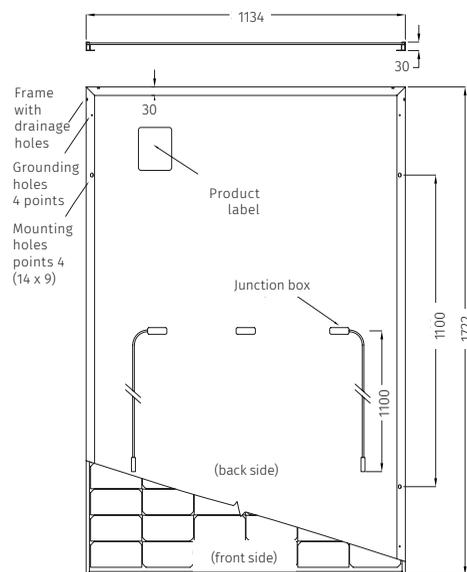
Note: dimensions in mm, tolerance +/- 2 mm
