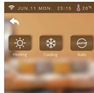
**Note:** Enter the password "168" in "Parameter" and set the heating & cooling type by modifying N02.
